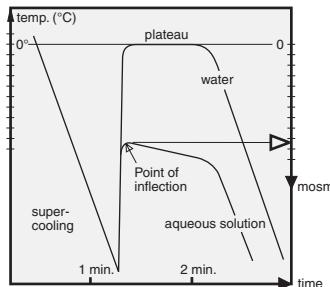
with an osmolality of 1 osmol / kg water at  $-1.858^{\circ}\text{C}$ . 1 Mol of a substance dissolved in 1 kg of water gives a solution with an osmotic concentration of 1 osmol / kg water only if it is an ideal solution and if the substance does not dissociate.
